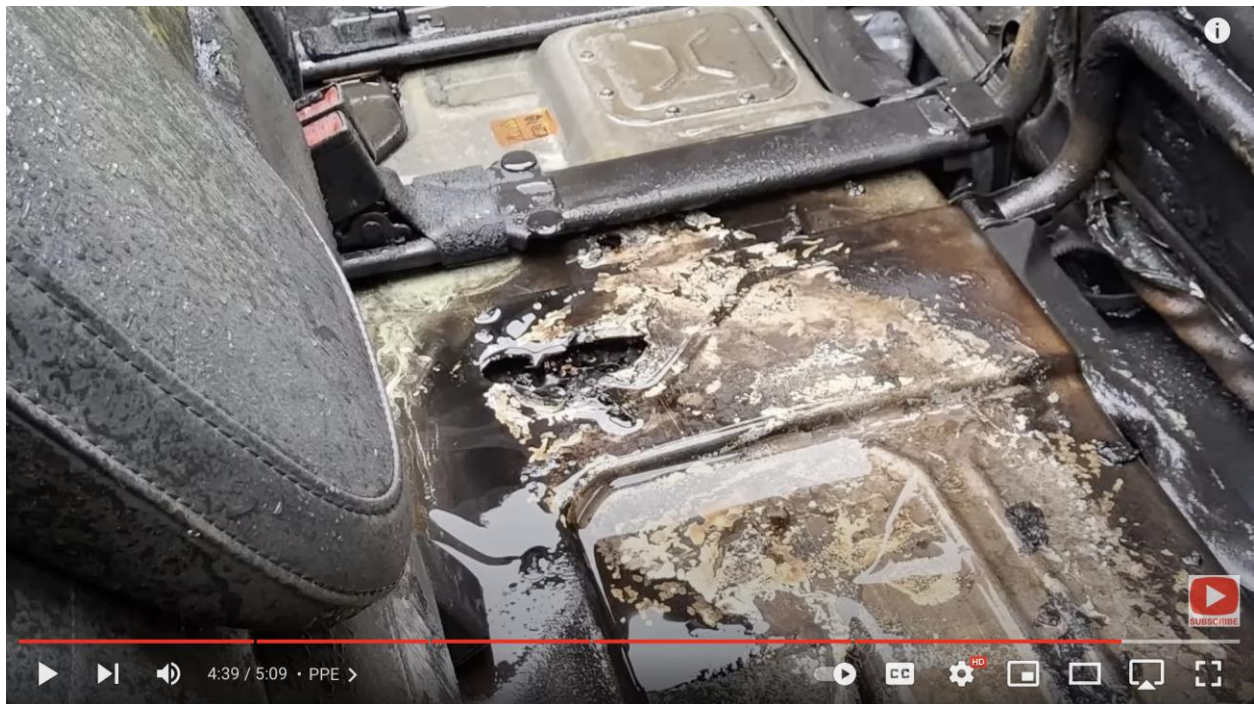
Image of the HV Battery After October 30, 2023 Explosion of Jeep Wrangler 4xe in Belgium
